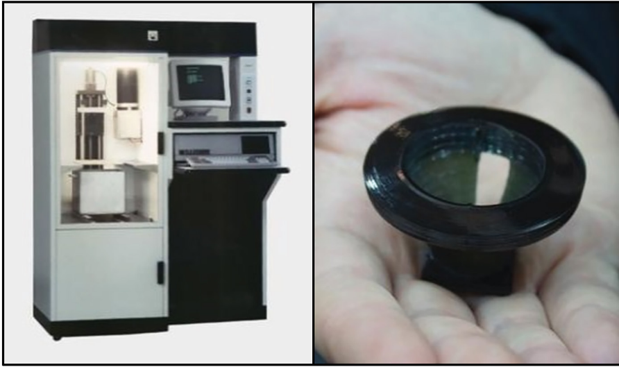
Figure 1.1 First Stereolithography Machine and First 3D Printed Part
