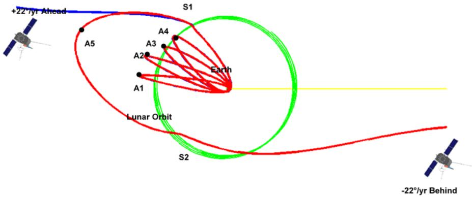
**Fig. 5** Illustrated are the phasing orbits of the two observatories. Observatory A was ejected into heliocentric orbit after spending 52 days in Earth orbit. Observatory B re-encountered the Moon 38 days later and was ejected into a trailing orbit
