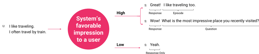
Fig. 1 Main idea of the proposed system that selects the next system utterance based on the system’s favorable impression toward the user (U: user, S: system)
