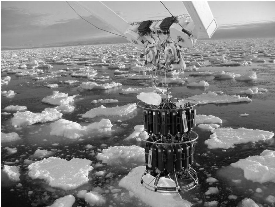
Figure 2.1. Chassis equipped with 28 seawater sampling bottles, a CTDO 2 probe and acoustic Doppler current meters. The bottles are closed on the upcast at depths chosen to sample the different water masses. East Greenland Plateau at 60°N in June 2002 (©OVIDE/Ifremer)
