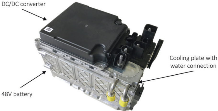
Fig. 3. The 48V powerpack at the heart of powernet systems integration
