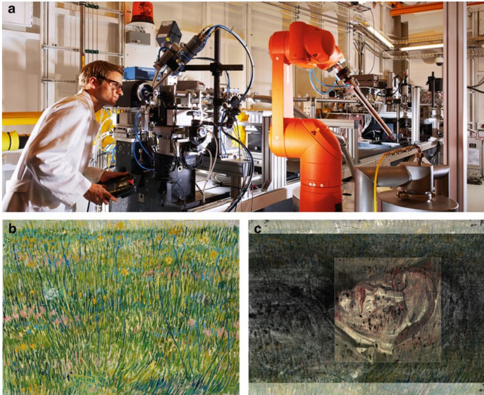
Fig. 2.2 (a) Experimentierstation P11 bei PETRA III (courtesy of © DESY). (b) Vincent van Gogh, Patch of Grass. Painted over one of the 50 farmer's heads: Head of a woman (© Nuenen Collection Kröller-Müller Museum, Otterlo, the Netherlands. Reprint with kind permission). (c) The colored central part was reconstructed using synchrotron XRF scans, the b/w outer part by means of MA_XRF in situ. This visualization of the painted-away first painting became possible thanks to the University of Antwerp, TU Delft, DESY and the Kröller-Müller Museum (courtesy of © Nuenen Collection Kröller-Müller Museum, Otterlo, und University of Antwerp, TU Delft, the Netherlands. Reprint with kind permission)
