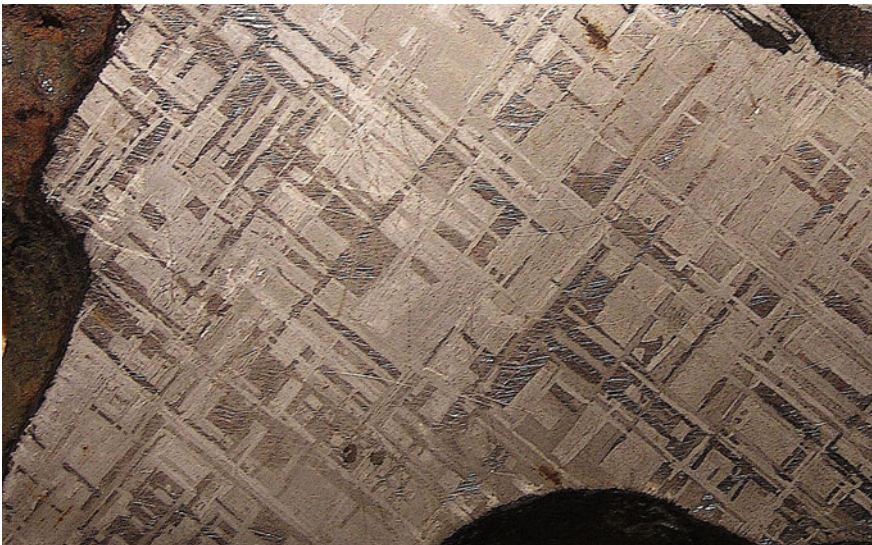
Fig. 1.2 Widmanstätten pattern made visible on an iron meteorite. The texture results from the intergrowth of the two minerals kamacite and taenite with different Fe/Ni ratios. Picture about 5 cm across
