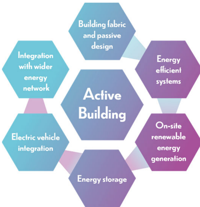
Fig. 5 Core principles of an active building [1]
