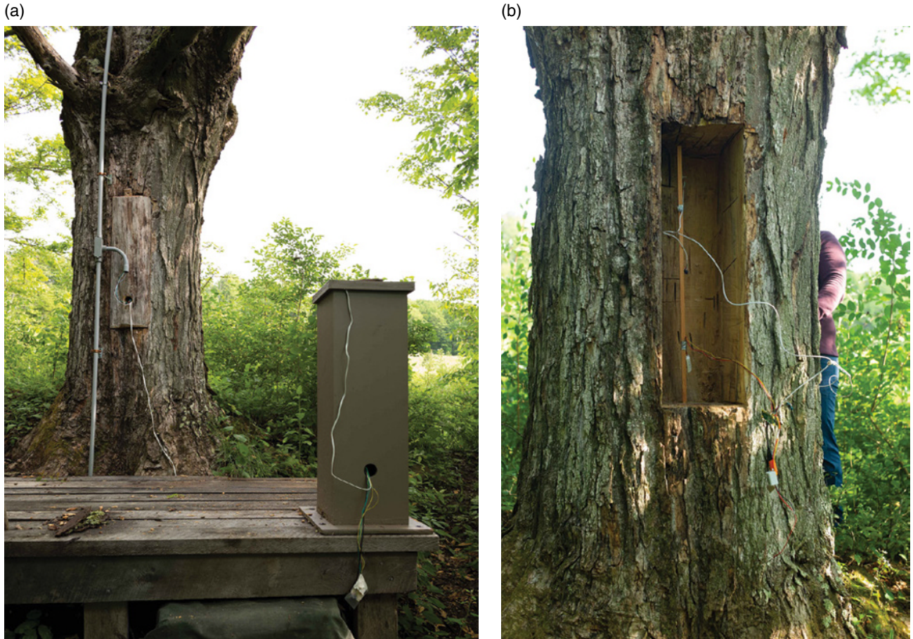
Figure 1.5 A research station beside the Shindagin Hollow State Forest in upstate New York. It was designed to test the environmental fluctuations – temperature ( ^{\circ}\text{C} ) and relative humidity (%) – inside two cavities of identical dimensions but with walls of different thicknesses, c. 2 cm vs. 20–30 cm. One (a) is a wooden box with walls like those of a Langstroth hive and the other (b) is a live sugar maple tree ( Acer saccharum ) in which a typical size bee cavity was cut using a chainsaw and adze. Source: Photo by Robin Radcliffe.
