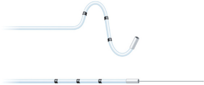
Fig. 1.16 Over-the-wire leads to facilitate placement in coronary vein branches. Top: lead with wire advanced beyond the distal end. The wire acts as a track over which the lead is advanced to provide stability. Bottom: lead with wire removed for final deployment.
