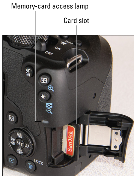
FIGURE 1-2: Insert the memory card with the label facing the back of the camera.
