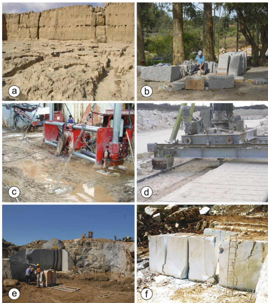
Fig. 2.2 Methods of stone exploitation from the past to present: (a) prehistoric traces of the use of wood edges to cut the stone (Egypt, Giza), (b) manual splitting of granite in Uruguay, (c) drill hole aided extraction, (d) the use of a saw for the extraction of soft porous limestone (Sósút, Hungary) (e) in-situ gang-saw cutting for stone extraction in the dolerites in Uruguay and (f) reducing the block size at the quarry level (Thailand)
