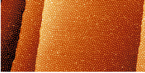
Fig. 1 155 \times 108 \text{ nm}^2 STM topography of a Ag(111) surface covered by 1% ML of Ce adatoms at a temperature of 3.9 K ( U_s = -90 \text{ mV} , I_s = 40 \text{ pA} ). Nearest neighbor adatom-adatom separations are 3.2 nm. Dark ( bright ) contrast: lower ( upper ) terrace separated by a monatomic Ag step. After Ref. [4]
