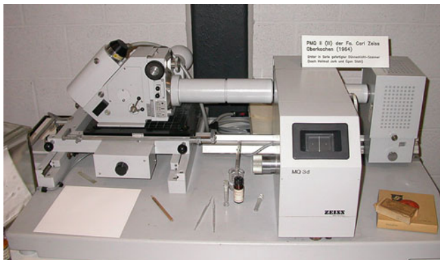
Fig. 1.5 The first TLC scanner (ZR3), constructed by Jork for Zeiss, Germany [45]
