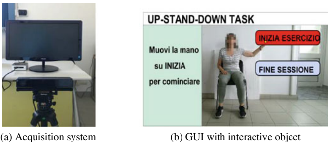
Fig. 1 a The vision-based system consisting of RGB-Depth camera, mini-PC and monitor. b Example of GUI with interactive objects to perform selections
