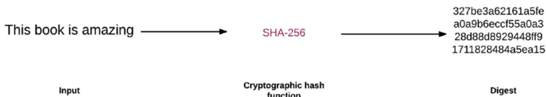
Figure 1-2. Mechanism of a cryptographic hash function. It takes an input and consistently converts it to a string of an output digest
