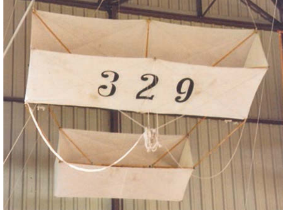
Fig. 1. Kite used by the meteorological observatory in Lindenberg, Germany, for meteorological measurements throughout the whole troposphere at the beginning of the 20th century.
