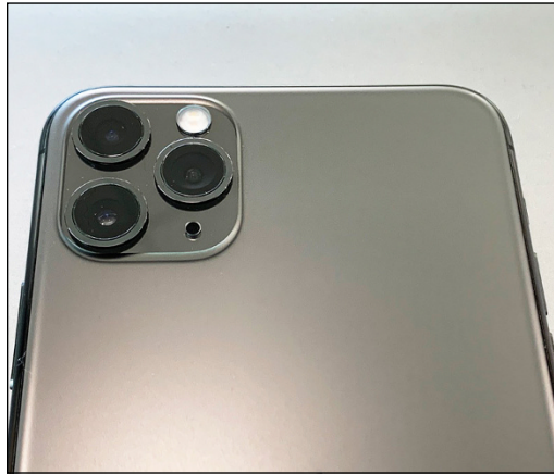
FIGURE 1-3: Triple lens cameras that come with the iPhone 11 Pro and 11 Pro Max models.
