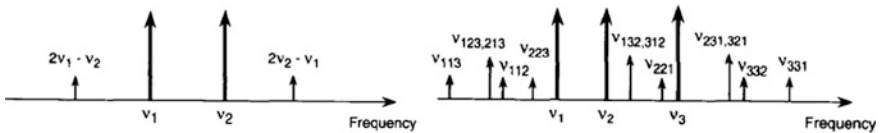
Fig. 9 Schematic diagram of four-wave mixing effect for two-channel and three-channel WDM systems
