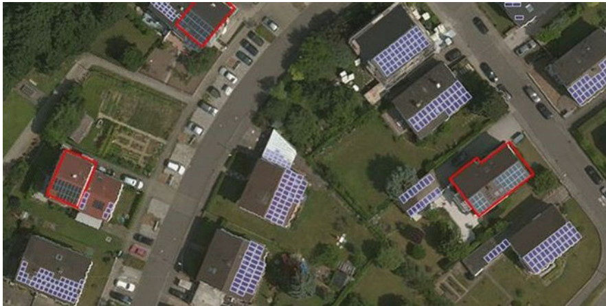
Fig. 2 Possible module placement for new PV systems with lowest possible electricity production costs (blue/white) and roofs that are already covered with PV modules (red border). Own depiction with map data from Bing Maps [2]
