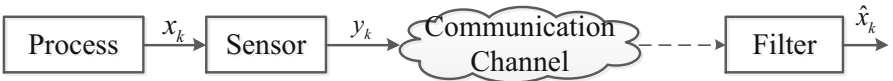
Fig. 1.4 The system diagram of intermittent filtering, the performance of which is mainly affected by the communication channel
