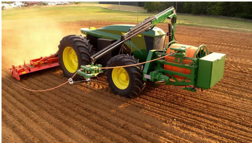
Fig. 1. The all-electric, fully autonomous GridCON Tractor.
