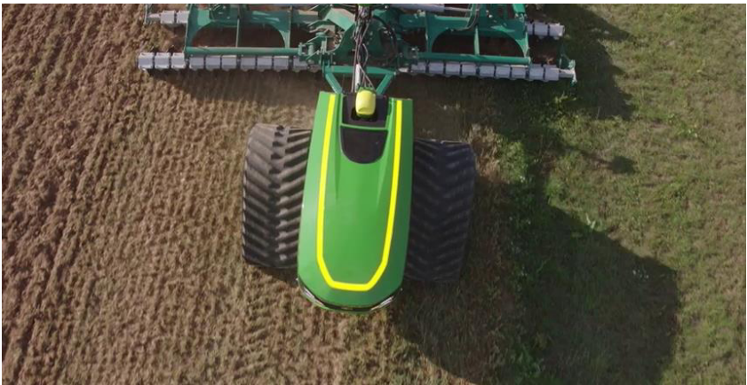
Fig. 6. Swarm Unit actively steering to perform field work with a pure pursuit based lateral path tracker during preliminary tests.
