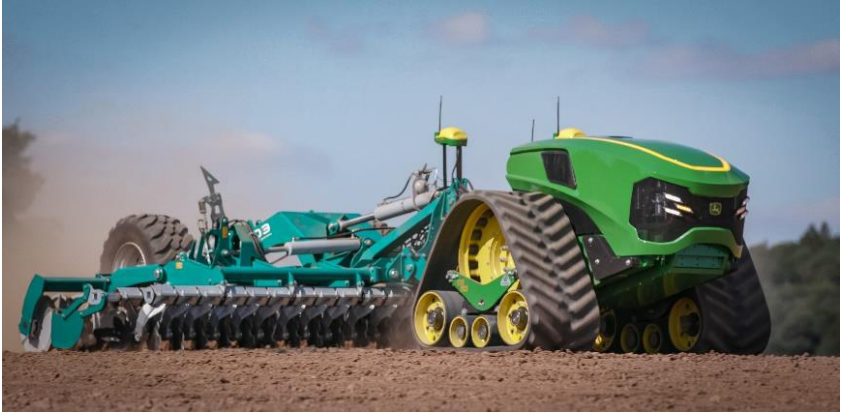
Fig. 2. The all-electric, fully automated swarm unit [6].
