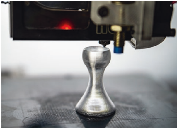
Figure 1-1. A 3D print in progress
