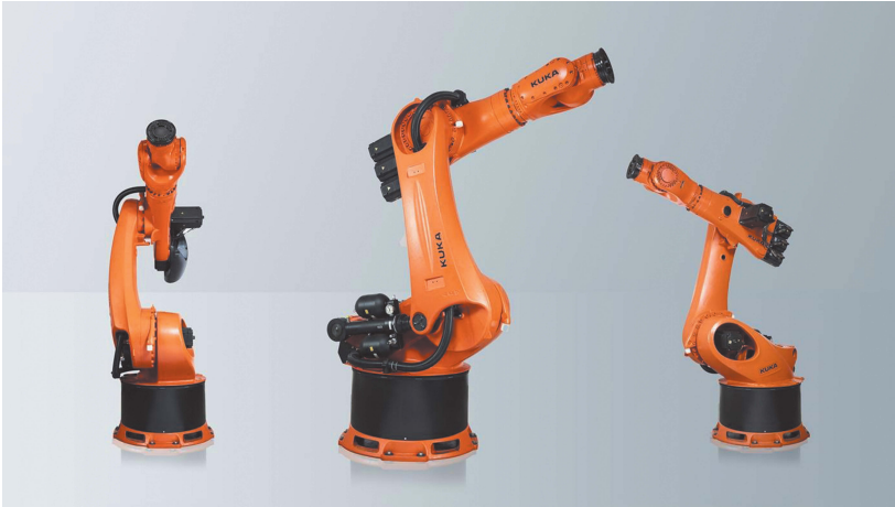
Figure 1.1: A six-axis industrial manipulator, the KUKA 500 FORTEC robot. (Photo courtesy of KUKA Robotics.)
