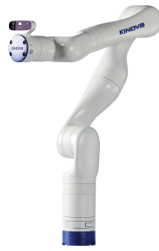
Figure 1.5: The Kinova ® Gen3 Ultra lightweight arm, a 7-degree-of-freedom redundant manipulator. (Photo courtesy of Kinova, Inc.)
