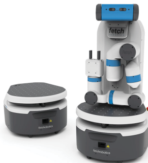
Figure 1.3: Example of a typical mobile robot, the Fetch series. The figure on the right shows the mobile robot base with an attached manipulator arm. (Photo courtesy of Fetch Robotics.)
