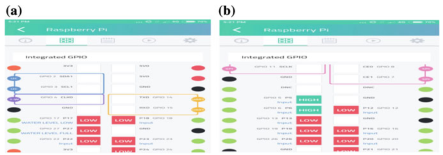
Fig. 3 a, b Raspberry PI connections being configured through the Cayenne app
