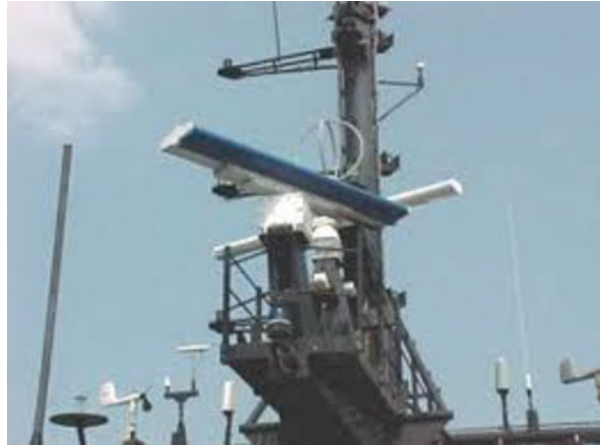
Fig. 1.15 Navigational radar cruise system
