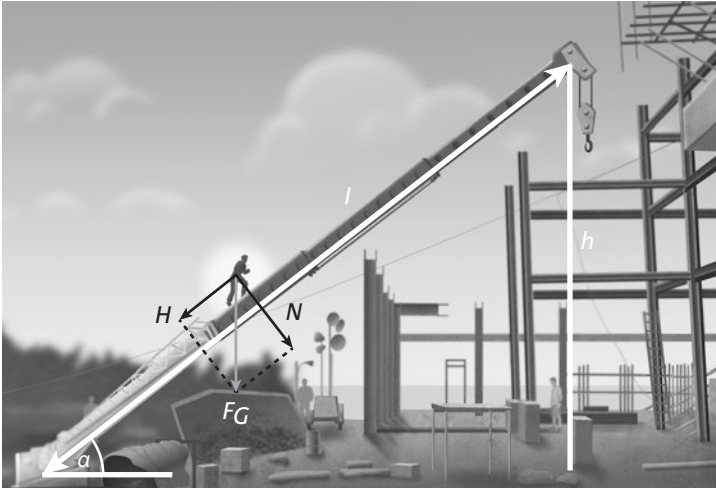
Figure 2.2 James Bond can reach a construction site by walking up the boom of a truck-mounted crane. In the picture are shown the height h and length l of the boom as well as the parallel H and perpendicular, or normal, N force-components of Bond's weight force F_G . The angle of attack of the boom is \alpha \approx 40^\circ
