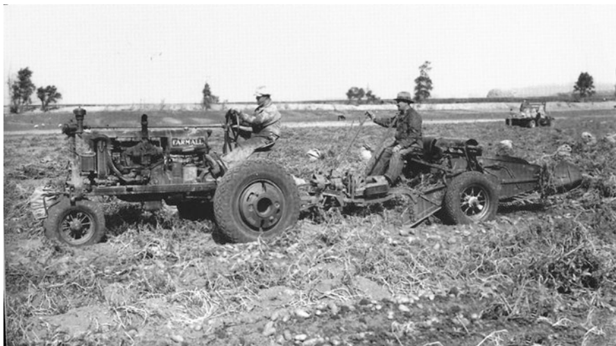
Fig. 1.13 Early generation tractor and single row potato harvester. (Public domain image from Wikimedia Commons)
