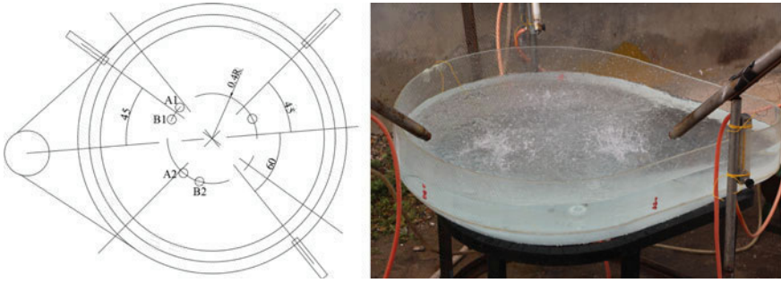
Fig. 2 The combined blowing arrangements in EAF model
