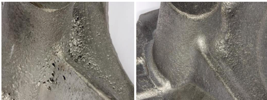
Fig. 7. Porosity on the casting (left) and after forging (right)
