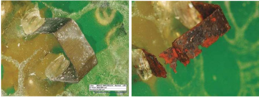
Fig. 1.24 A SWA corrosion sensor removed from a concrete block had an un-corroded sacrificial metal link sensor strip (left) and a corroded strip (right) (photos courtesy of FDOT)
