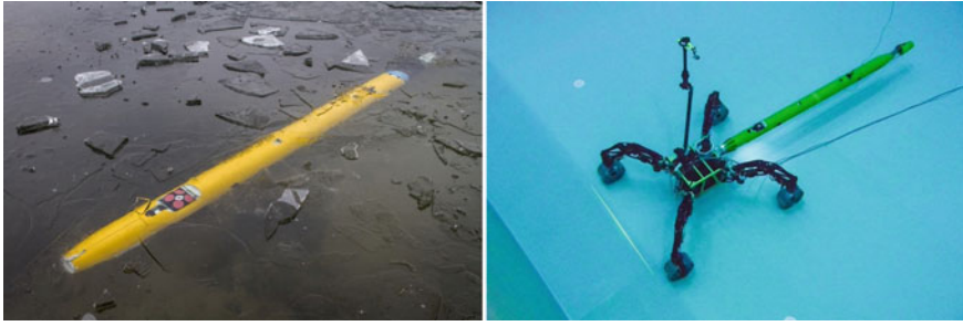
Fig. 7 The Underwater Robot Leng. The system is actually a study to explore the depths of extraterrestrial oceans (study for the german space administration) but has been used here to simulate multi robot scenarios. The right picture shows the robot Leng docking to the robot Sherpa-UW in an attempt to exchange huge amounts of data, which is inefficient to do via radio link in water
