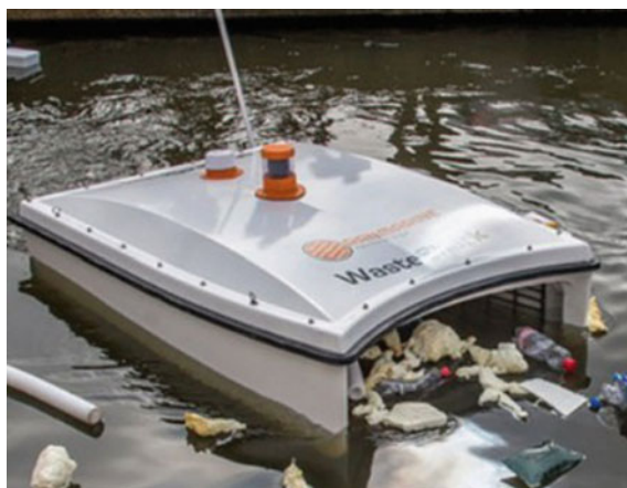
Fig. 2 The Waste-Shark. A study of an autonomous robot to collect floating waste in harbours and other confined maritime environments
