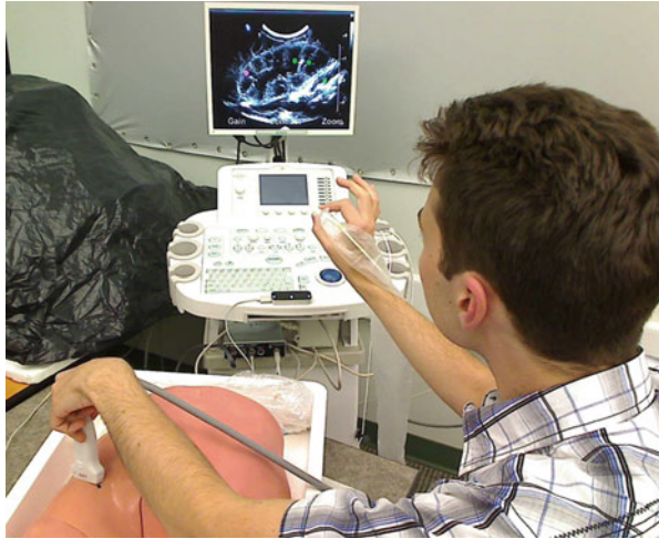
Fig. 2 A hand gesture tracked interface for controlling an ultrasound workstation
