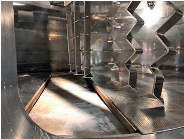
Figure 1.5 A peek into the lauter tun at Urban Village Brewing Company. Source: Photo: Dave Goldman.
