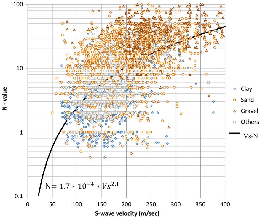
**Fig. 1** Correlation between S-wave velocity and N-value obtained from standard penetration tests at many Japanese levees with soil classification. S-wave velocities were obtained by a surface wave method performed on the levee surface. The black line is a regression line obtained by the least squares method
