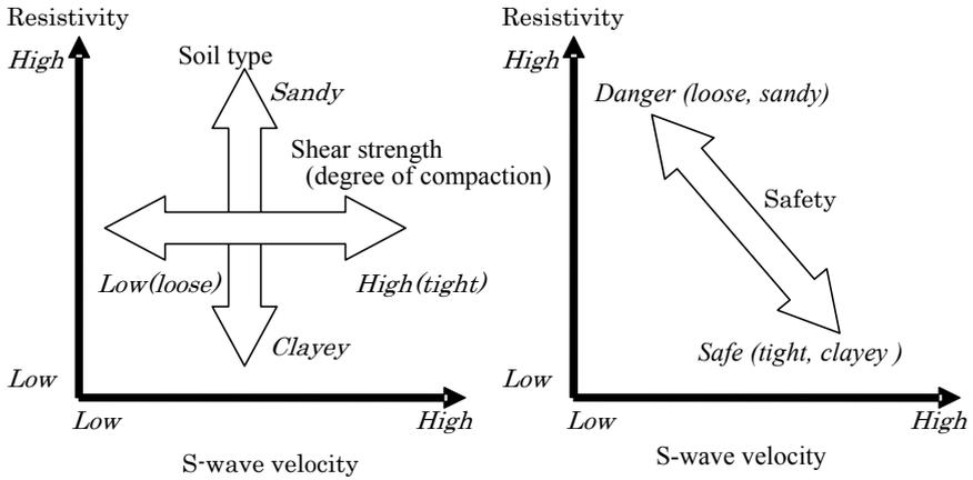
**Fig. 3** Schematic relationship between geophysical properties and soil condition (left) and levee safety (right). The left figure shows a schematic relationship between S-wave velocity and resistivity. The right figure shows a schematic relationship between geophysical properties, S-wave velocity and resistivity, and the vulnerability of levees
