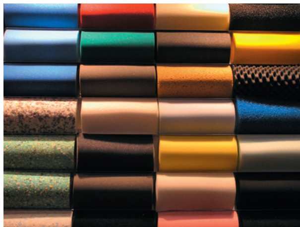
Figure 1.6 Polyurethane can exist as both a thermoset and a thermoplastic. It can also be rigid or soft as seen in the foam blocks shown here.
