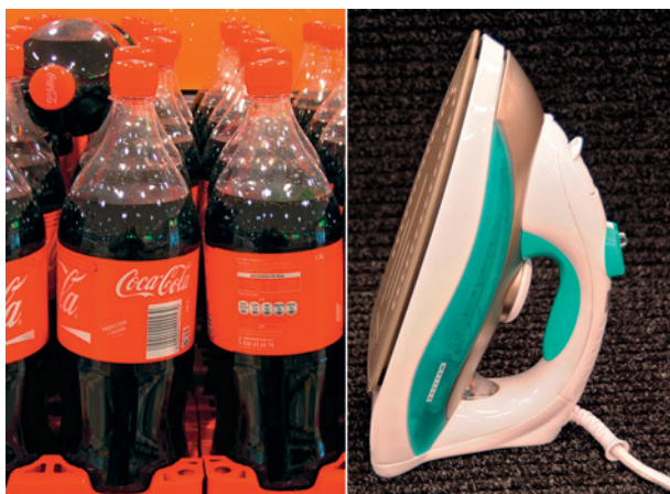
Figure 1.9 Thermoplastic polyester (PET) is a plastic that can be either amorphous, as in soft drink bottles, or semi-crystalline, as in the iron.
