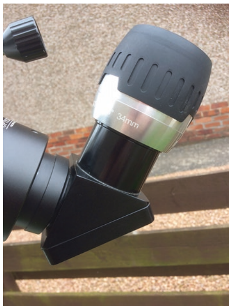
Fig. 1.3. The ShortTube fitted with a 34-mm wide angle eyepiece yielding an enormous 5.8 degree true field. (Image by the author.)
