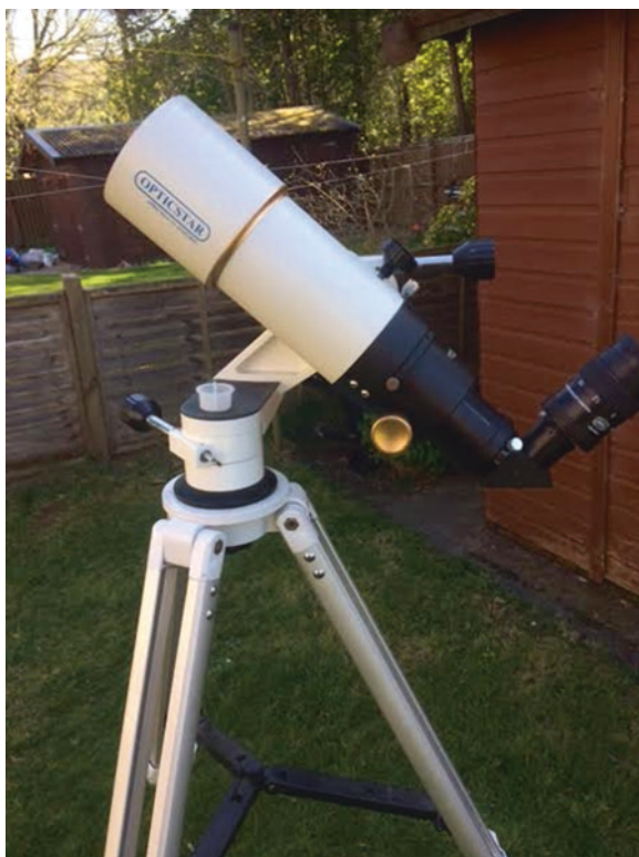
Fig. 1.2. The ShortTube 80 is a fine ultra-portable ‘scope seen here mounted on a Vixen Porta II Altazimuth Mount. (Image by the author.)
