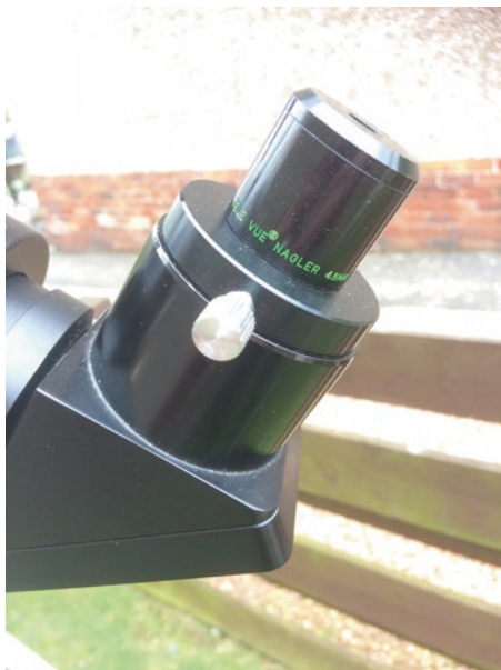
Fig. 1.4. A little 4.8-mm T1 Nagler serves as a great higher power eyepiece for the ShortTube 80. (Image by the author.)
