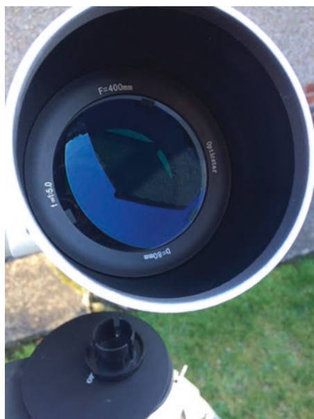
Fig. 2.1. The air-spaced doublet objective of the ShortTube 80. (Image by the author.)
