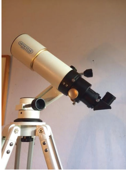
Fig. 2.2. The Standard ShortTube 80 usually comes equipped with a 90-degree 1.25” mirror diagonal much like the ones shown in the image. (Image by the author.)
