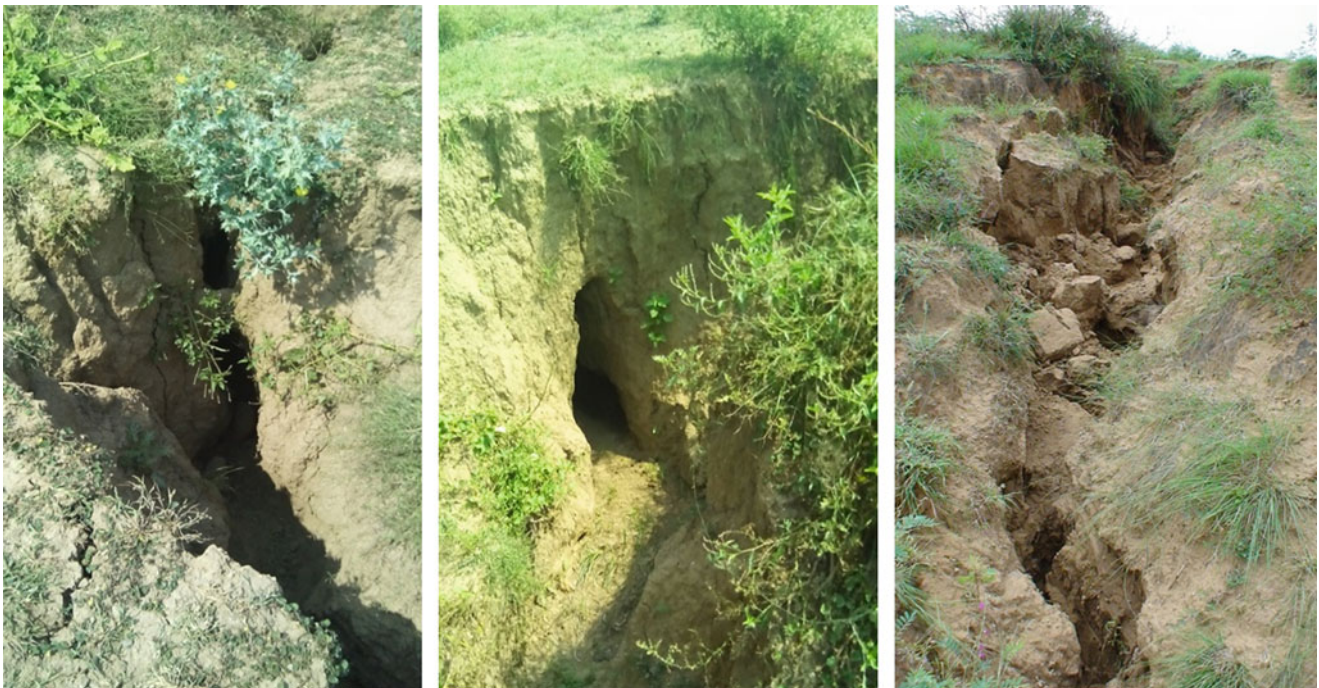
Fig. 1.5 Tunnelling as observed on adjacent tableland near ravine and on bank slope
