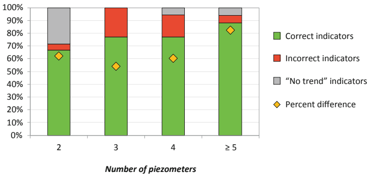
Fig. 3. Influence on the correctness of the results of the numerosity of piezometers
