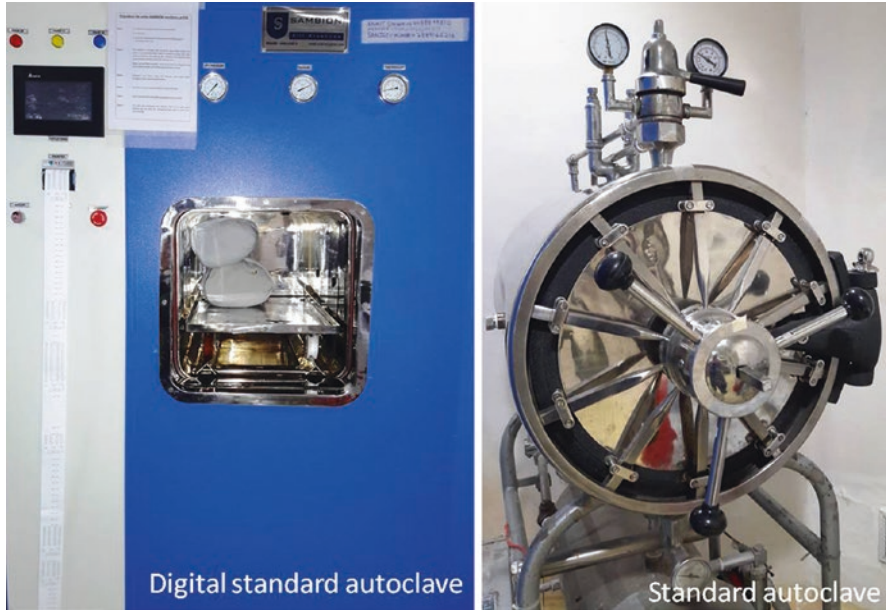
Fig. 1.3 The digital autoclave containing wrapped linen with the autoclave cycle parameters and timings recorded on a printed strip. The standard autoclave shows analogue gauges and meters with no record of previous cycles.
