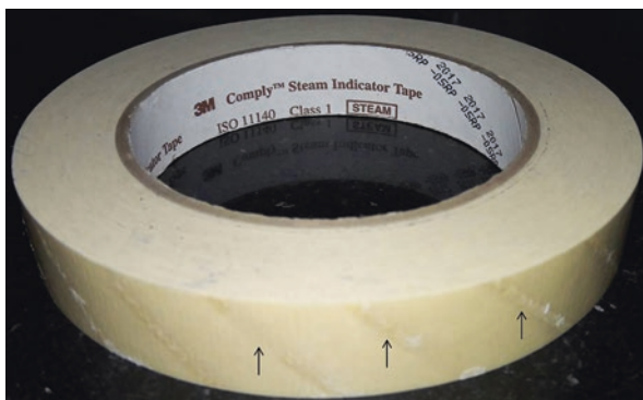
Fig. 1.5 A steam indicator (chemical) tape with the arrows showing the site of chemical stripe. The space in between two lines is used to label the date, time and signature of nursing officer
