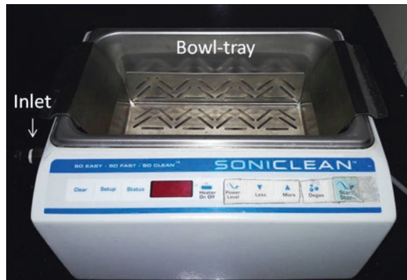
Fig. 1.1 An ultrasonic cleaner with a bowl-tray to contain the instruments to be cleaned. The arrow highlights the 'inlet' for the water or solution
