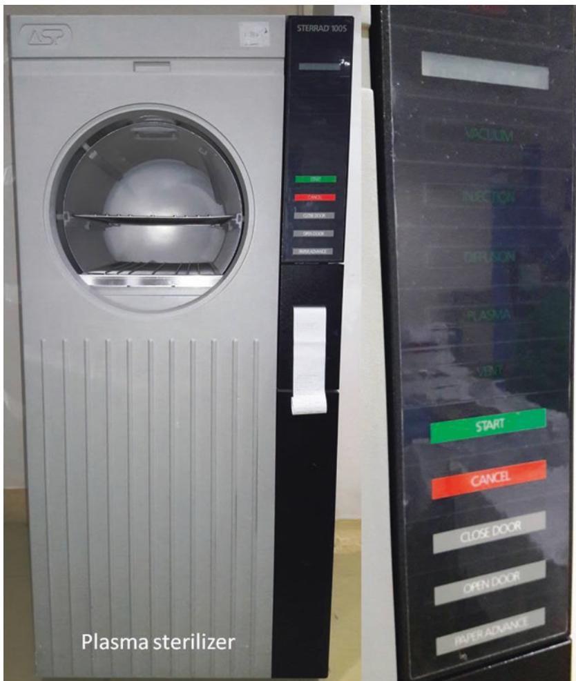
Fig. 1.4 The plasma sterilizer with 'open door' showing the shelves to keep the wrapped items. Each cycle is printed on the stripe for record maintenance. Various options and cycle stage indicators
