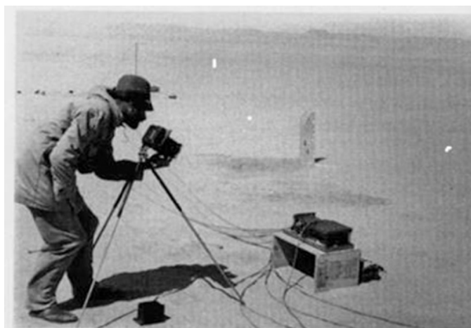
Wind measurements being made with my multiple manometer in a sand storm near Gilf Kebir, 1938. The sand collector is in the middle ground. Photograph by Ronald Peel.
