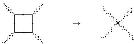
Fig. 3. The one-loop diagram of QED is replaced in the effective theory by 4-photon contact interactions.
