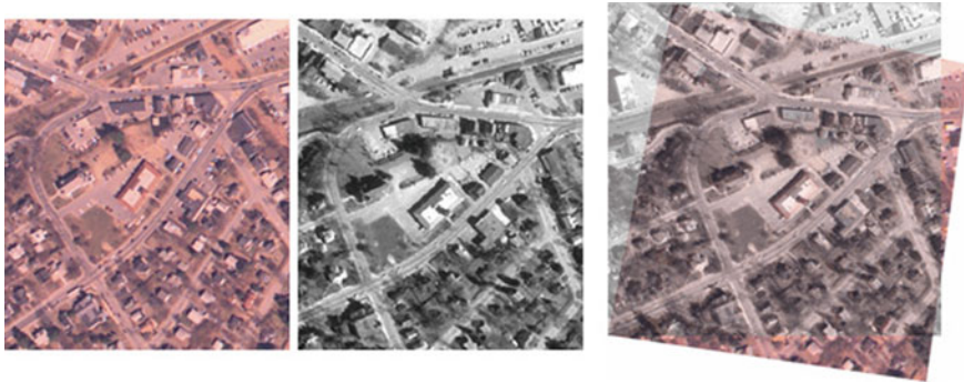
Fig. 1.2 Another sample that can be taken as an example for multi-view image registration; first two are the aerial shots of a single scene at different angles, third is the registered image. (A digital aerial photograph [geometrically uncorrected] to a digital orthophoto [supplied by the Massachusetts Geographic Information System (MassGIS), has been orthorectified] covering the same area centered on the business district of West Concord, Massachusetts, USA https://in.mathworks.com/discovery/image-registration.html )
