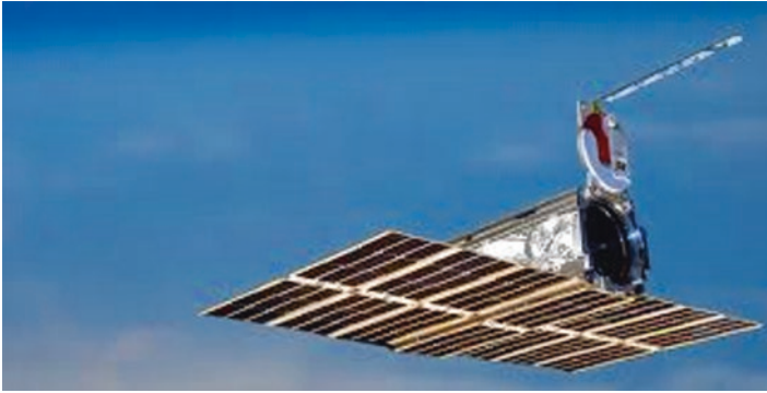
Fig. 1.2 A Dove 3-unit cube sat, about the size of a small bird. (Graphic courtesy of Planet.)
