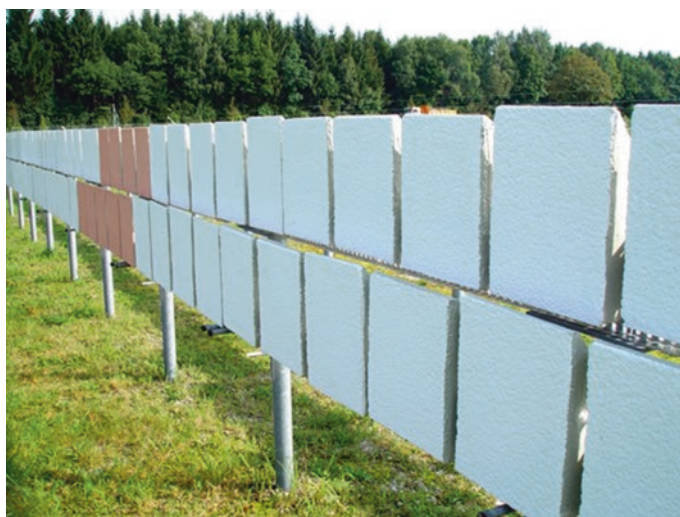
Fig. 2.2 Exposition of the specimens at the main location in Valley/Holzkirchen shortly after the start. Above the specimens, bird protecting threads can be recognized (Hofbauer et al. 2006; Hofbauer 2007)
