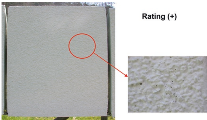
Fig. 2.6 Rating scale level + with detail of observed growth (Hofbauer et al. 2006; Hofbauer 2007)
