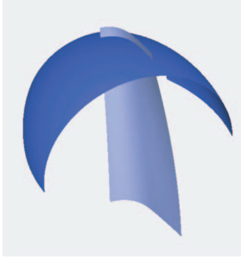
Fig. 1.1. Transversal intersection between two sculptured surfaces
