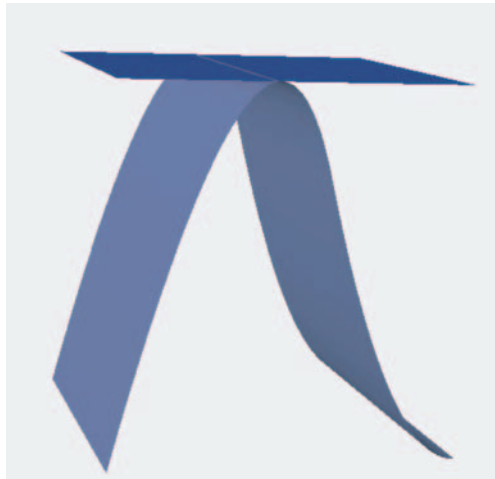
Fig. 1.2. Tangential intersection between two surfaces
