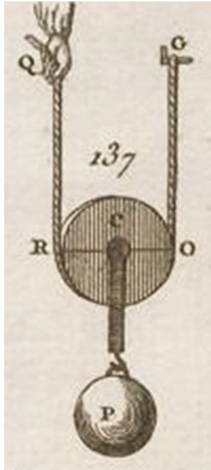
Fig. 10. A fixed pulley in Bézout.
