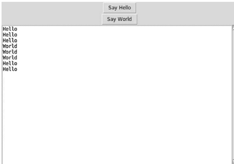
Figure 1-1. Our Tkinter GUI application after a series of clicks of “Say Hello” and “Say World”
