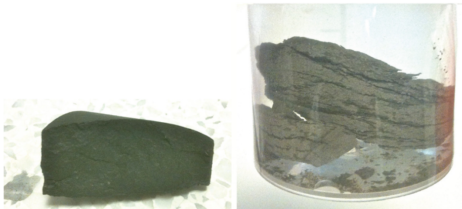
Figure 1.6 Opalinus Clay preserved (left) and the same sample after a few seconds in a non-appropriate brine solution (right); note the massive structural deterioration.
