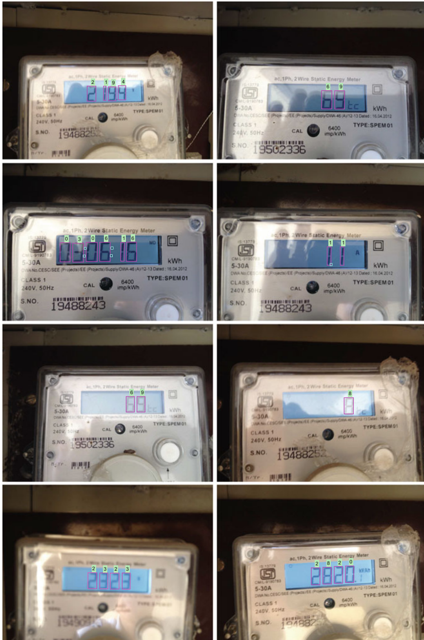
Fig. 5 Representative results of the proposed method. The segmented digits are represented in terms of the bounding boxes and the corresponding recognized results are overlaid above each digit. The method can handle images exhibiting uneven illumination, the presence of shadows, poor contrast, and blur
